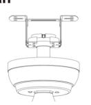
☐ Lift the fan motor assembly up to the mounting bracket and seat the hanger ball in the mounting bracket socket. Rotate the fan motor assembly until the check groove drops into the registration slot and seats firmly. The downrod should not rotate if the is done correctly
