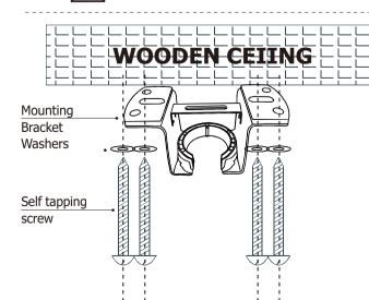
For wooden ceiling, use wood screw to drill on the wooden beam or the "junction box" to fix the hanging bracket(selection is made according to actual requirements of the customers)
