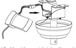
1. Carefully push the canopy to the bottom of the mounting bracket, make two sliding holes aligned to the two prominent screws on the mounting bracket, and then turn clockwise 2. Push the canopy ring to the bottom oft he canopy, slide the inner holes aligned to the two prominent screws on the mounting bracket again, and turn the canopy ring
