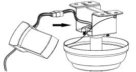
1. Carefully push the canopy to the bottom of the mounting bracket, make two sliding holes aligned to the two prominent screws on the mounting bracket, and then turn clockwise 2. Push the canopy ring to the bottom oft he canopy, slide the inner holes aligned to the two prominent screws
