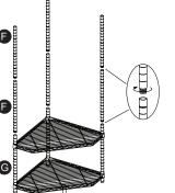
6. Screw top pole (E) onto middle pole(F), hand tighten.
