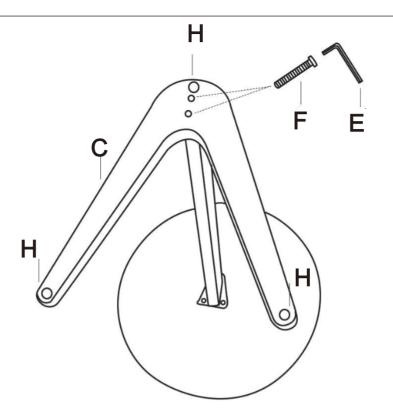
**Step 3**: Connect the Base [ C ] and the Bracket [ B ] with Two Screws M6\*35 [ F ] by Allen Wrench [ E ]. And paste the foot pad [ H ] to the bottom of base.
