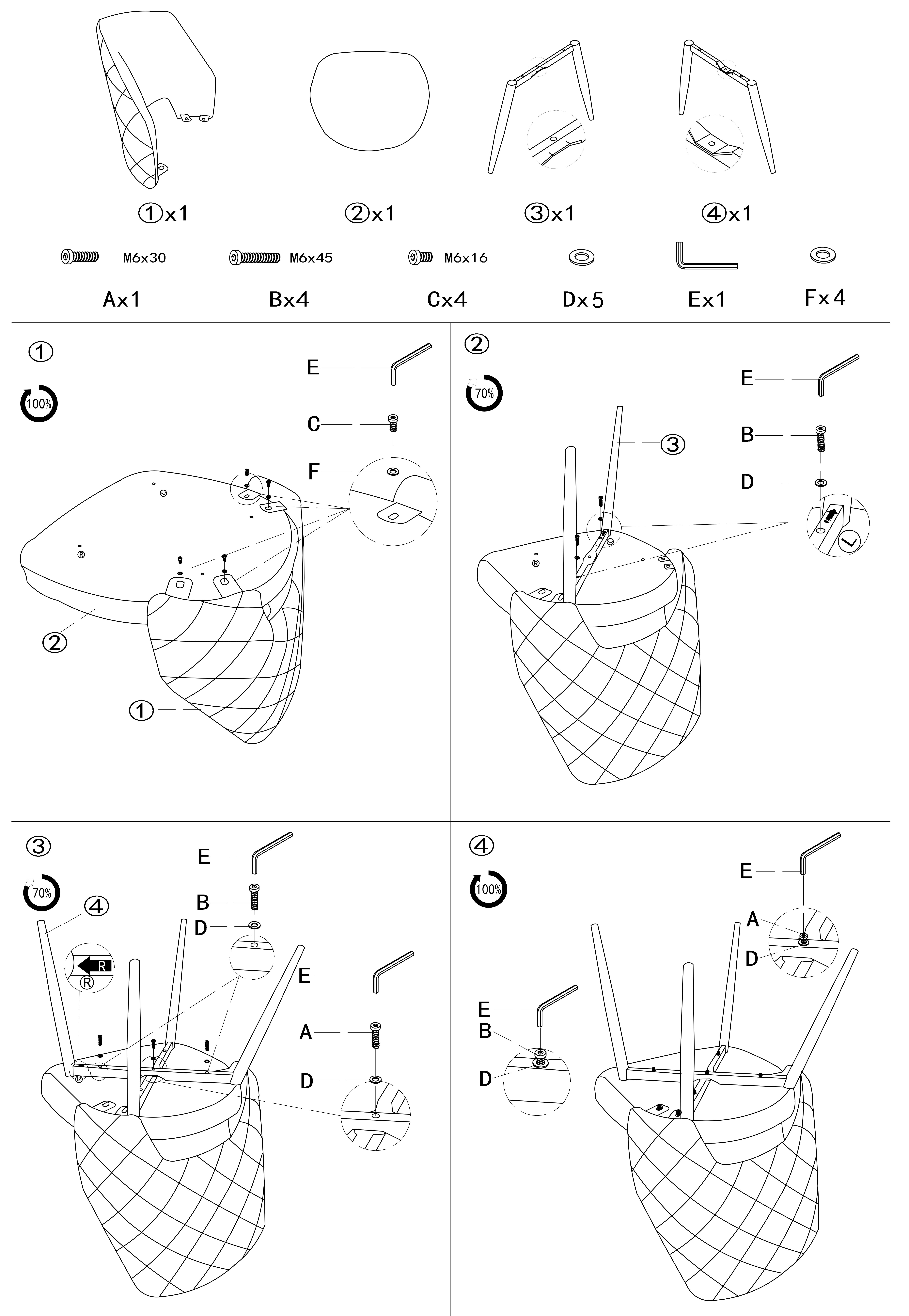
Tighten all the screws to 100% of maximum tightness
