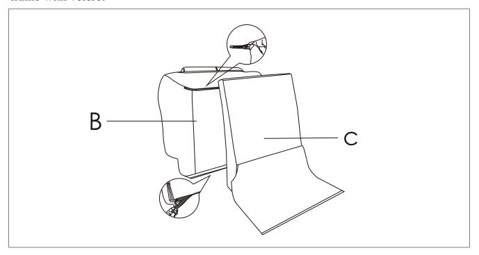
STEP10:Plug the back pad into the seat frame, and then connect the massager line white and white, red and red, black and power lines, and the massage line with the hand controller.
