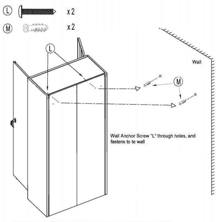
AFTER ASSEMBLLY IS COMPLETE, THE UNIT MUST BE SECURED TO A WALL. FAILURE to mount the unit to a wall, can create a TIPPING HAZARD. A tipping hazard is dangerous to yourself and others. Use wall anchor hardware that properly suits the installation of mounting this unit to a wall
