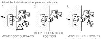
by turning this screw counter-clockwise
