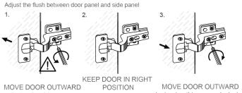
by turning this screw counter-clockwise
