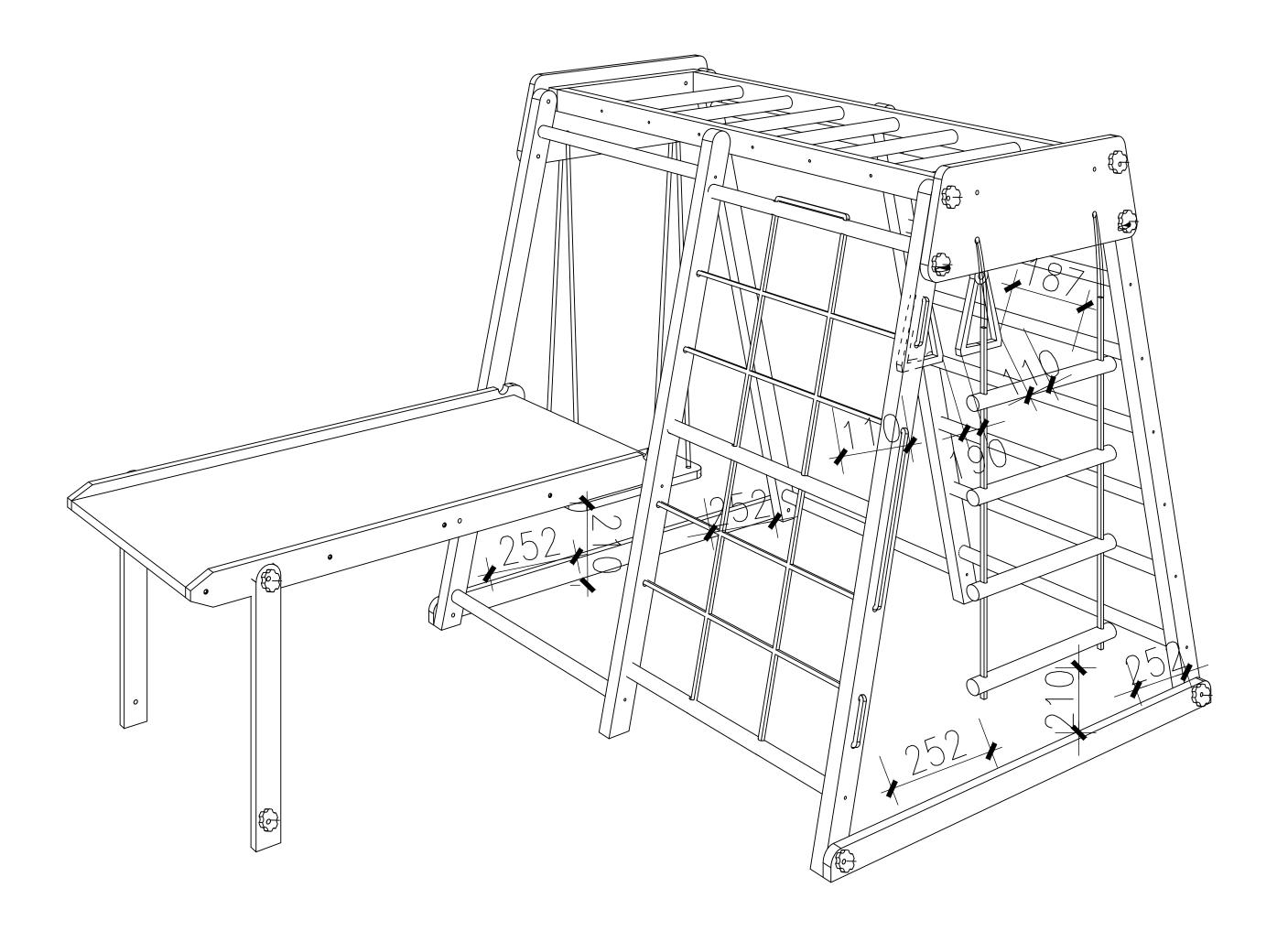
Note: The length of the grid climbing rope is 6.45 meters, the soft ladder is 3 meters long, the pull ring is 1.4 meters long, and the swing rope is 4 meters long. All ropes are the same, minimum diameter of rope: 10mm.
