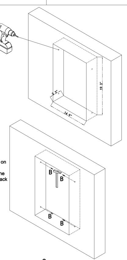
Mark four (4) mounting holes on the wall corresponding to the pre-drilled hole lo cations in the mounting bars on theinside back panel of the cabinet.
