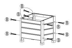
Assemble front panel of storage box, back panel of storage box, left panel of storage box and right panel of storage box.
