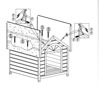
Assemble the roof and left and right braces.
