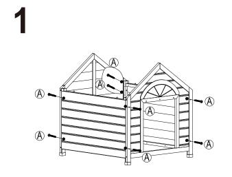
Assemble front panel, back panel and side panels.
