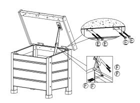
Assemble storage box roof and right brace.
