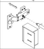
If the door gap is large,you can adjust the hinges left and right
