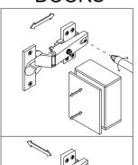
If the hinge holes are notaligned, you can tryadjusting the front and rear hinges.
