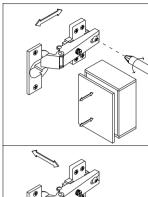
If the hinge holes are notaligned, you can tryadjusting the front and rear hinges.
