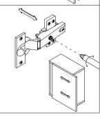
If the door gap is large,you can adjust the hinges left and right
