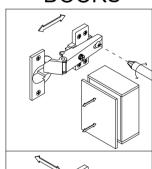
If the hinge holes are notaligned, you can tryadjusting the front and rear hinges.
