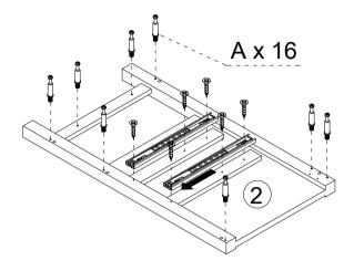
The slide rail can be pulled out in this direction
