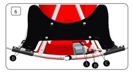
Turn over the vehicle body, you can see there are connectors on A, B, C and D
