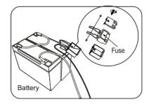
The vehicle is equipped with a self-resetting fuse. When the vehicle is overloaded or operated incorrectly; the self-resetting fuse will be cut off for 5-20seconds before becoming operational again. The self-resetting fuse is under the seat (Refer to the picture.)
