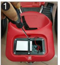
1.Remove the battery cover and all the screws.
