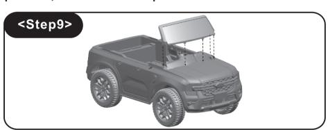
9.Insert the windshield in the front of the body,make sure it is firmly fixed.
