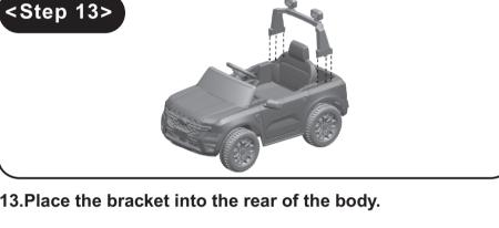
13.Place the bracket into the rear of the body.
