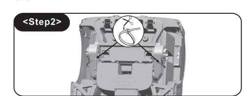
2. Turn over the body and find the gearbox, then cut the ties.
