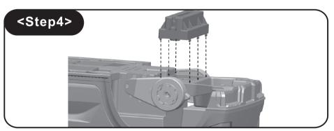
4. Place the rear support into the position of the body, make sure it is firmly fixed.
