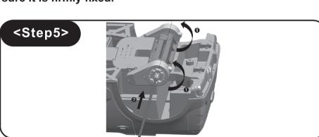
5. Rotate the gearbox and make the hole alignment, then insert the rear wheel axle.
