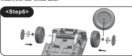
6.Insert the two wheels first and tighten with two nuts by the tools provided, then cover the wheel caps.
