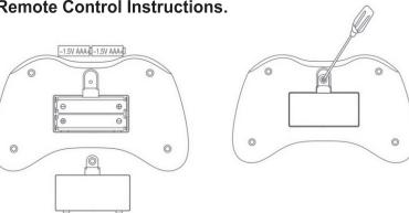
Loosen the screw with a screwdriver, and put 2 AAA batteries into the battery house. Cover with a battery cover and tight with a screw
