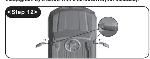
12. Place the two rear mirrors into the position of the body.
