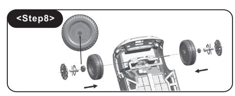
8.Insert the two front wheels and tighten two nuts by the tools provided, cover the wheel caps.
