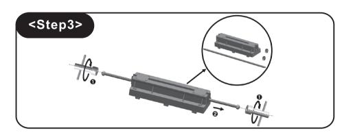
3. Release the two nuts with the tools provided, and pull the wheel axle out.
