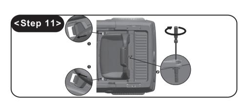
11.Place the front of the seat first, then close the rear of the seat,tighten by a screw with a screwdriver(not included).
