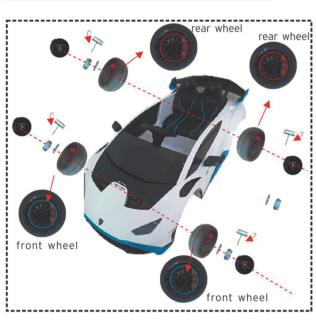
Install "4": Unscrew the gasket and nut from the axle:Insert "4". gasket and nut into the axle, then cover with "3".
