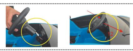
Install "1": connect steering wheel to column, lining up connectors "1" to "11", push the connectors into 11 slowly. "12" is buckle for fixing the steering wheel.
