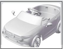
5. Install the reflectors Insert the reflectors into the grooves on the vehicle body as picture showed, make sure it is fixed.
