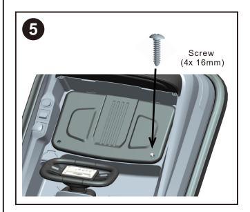
"Snap" the seat into the right place and fasten it with two screws(4 x 16mm) as picture shown.
