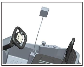
Charge the battery directly from the socket near the seat.
