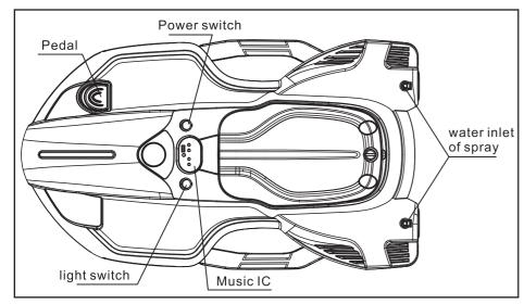
Open the power switch and step on the pedal switch, then the car moves forward. Release the pedal switch, the car will be stop.
