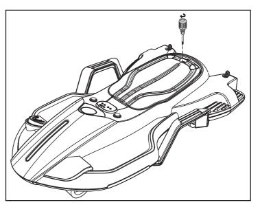
Open the seat locking buckle and two wire terminals are plugged in, then cole close the seat and lock the buckle, as pictures.
