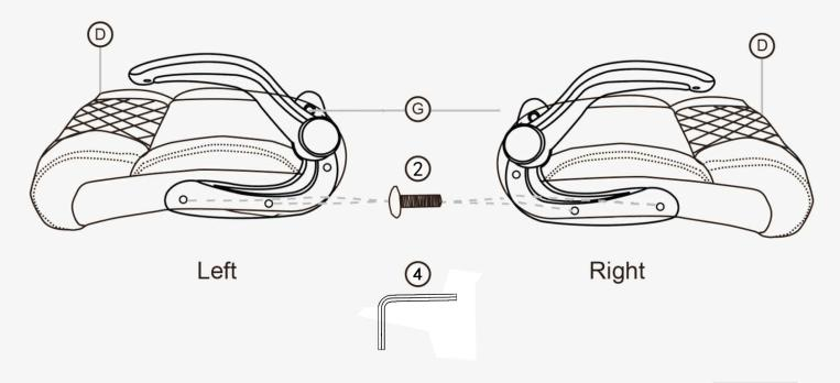
**STEP 5 :** Rotate the back of the chair up, then secure it with the top two M6\*35mm bolts.
