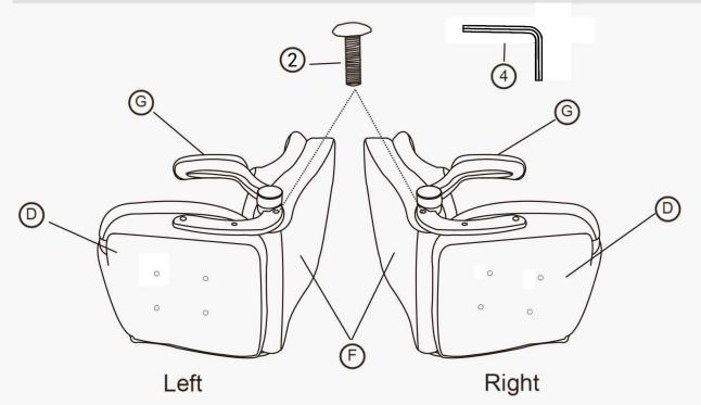
**STEP 6**:Align the seat plate to the bottom of the seat cushion, make sure that the front of the seat plate is facing the front of the seat cushion.Attach the seat plate to the seat cushion using four M6X25mm bolts, tighten all the bolts with the wrench.
