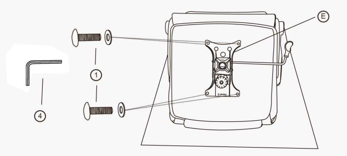
**STEP 7:** Turn the seat cushion upright and align the center hole of the seat plate over the lift, then push the seat cushion down onto the lift firmly until the connection is secure.
