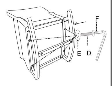
3.Attach the assembly from step 1 to the Seat Base using (4) M6x40mm Bolts (Part D) and (4) Φ18mm Washers (Part E), tighten with the M5 Allen Wrench(F).
