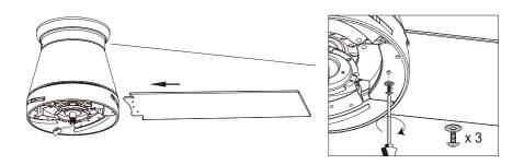
② Screw out the 3pc pre-installed screws from motor assembly,connect terminal.Then fix the light kit to the main body with screws.
