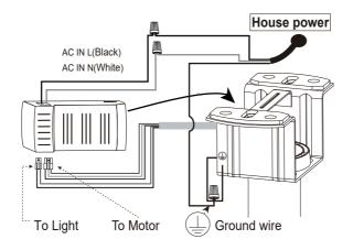
2 Put the receiver into the bracket and tidy up wires. Rotate the canopy counter-clockwise until screw heads engage the key slots fully. Tighten the screws. Be careful not to damage or cut the wiring.
