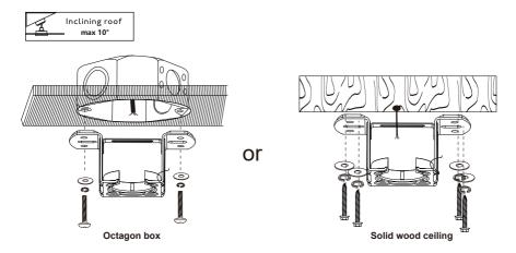
(3) Snap the basically assembled fan into the installed Bracket.
