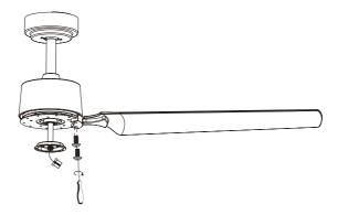
(2) Remove the pre-installed screws. Connect the light kit cable, and then lock the light kit.
