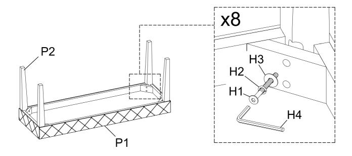
ADDITIONAL NOTE ABOUT SAFETY: BOLTS MAY LOOSEN DURING NORMAL EVERYDAY USE. THEY SHOULD BE PERIODICALLY INSPECTED AND RE-TIGHTENED TO PREVENT DAMAGE OR INJURY. ALWAYS CHECK TO BE ENSURE THAT ALL HARDWARE IS KEPT TIGHTENED.
