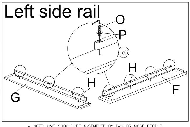
MOTE: UNIT SHOULD BE ASSEMBLED BY TWO OR MORE PEOPLE. DO NOT TIGHTEN ANY BOLTS UNTIL ALL BOLTS HAVE BEEN STARTED!
