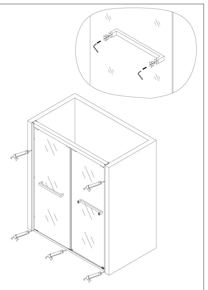
Apply silica gel to the walls and floors inside the shower room . Note: do not let water enter the door sealing strip directly. Wait 24 hours before using the shower.
