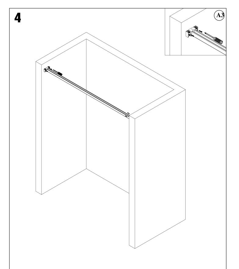
Put the anti-collision glue into the groove of the upper rail wall seat and tighten it to the wall with self tapping screws.
