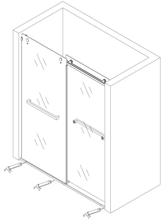
Apply silicone resin to the water retaining strip and floor at the bottom of the shower room.
