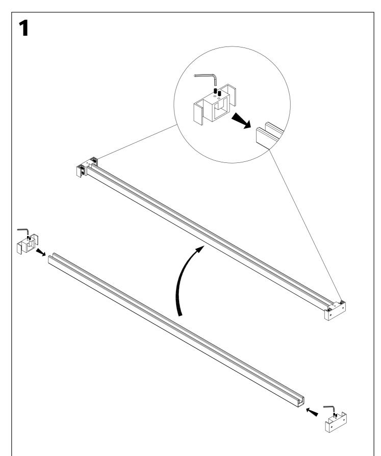
Install the wall seats at both ends on the upper rail before installation.
