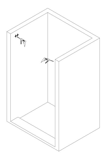
Drill holes according to the position marked in the previous step; Then knock the expansion pipe in at the position where the hole is drilled.
