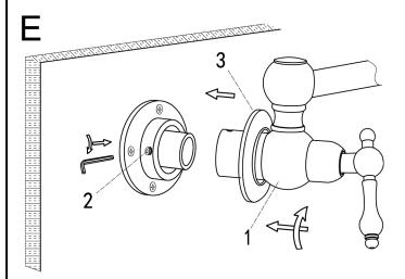
**5.** The decorative cover needs to be close to the wall, and the outlet is straight down after correct installation like the above figure.
