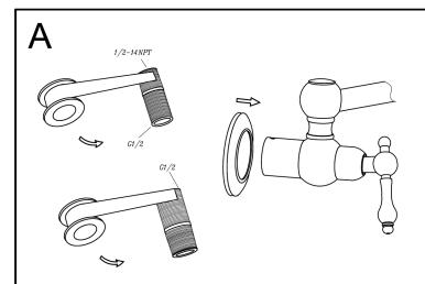
1. The thread which connecting the faucet to the pipe should be twined with Teflon tape to prevent water leakage.
