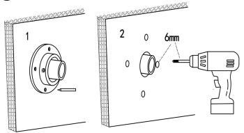
**3.** Cover the base on the inlet pipe and mark the four screw holes, then drill four holes in the wall to fix the screws.
