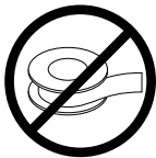
Pipe tape is not recommended.
