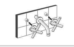
2. Mount the rough-in valve into its prepared location. Attach the valve body using the provided hardware. Use a level to ensure that the valve is mounted completely level.
