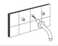
1. Prepare for installation by installing wood blocking between the two studs where the faucet will mount. The valve should be installed 2" behind the finished wall.
