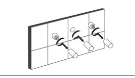
7. Attach the hot and cold handles by sliding them onto the left and right stems. Secure each handle by tightening the set screw on the bottom of the handle, using the provided hex wrench.
