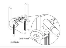
6. Attach the spout to the valve by twisting it into the middle valve outlet. Apply plumber's tape or a small amount of thread sealant to the threads before attaching.
