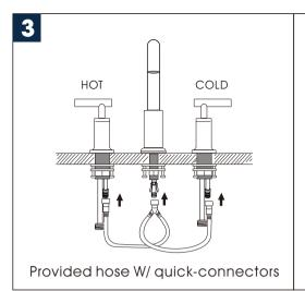
Align the position as shown, insert the quick-connector of the hose to the shank of the HOT/COLD handle and spout.
