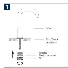
Insert the spout to the hole of sink/deck platform, align the washer, metal washer and nut as shown, thread the nut onto the shank and wrench tighten.
