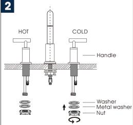
Insert the "COLD" handle on the right hole of the sink/deck platform, align the washer, metal washer and nut as shown, tighten the nut onto 'the shank by hands and tighten the screws to secure by tool. The "HOT"handle installation is same as "COLD"handle.
