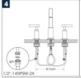
connect the water supplies. (Make sure washer is installed inside)
