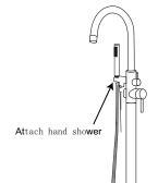
9. Once installation is complete, turn on the main water supply. Turn the faucet on and allow the water to flow for 60 seconds. Check for any leaks, and that hot and cold water are running appropriately. Divert the water to the hand shower and allow the water to flow through the hose for approximately 60 seconds
