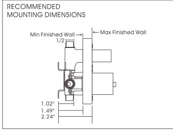
Connect the pipes into the valve body; Put valve body in the hole and fix it by the tapping screw. then connect the water supply hoses.
