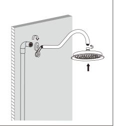
Roll the teflon tape on the thread of the shower seat. Tighten the shower seat clockwiseon the outlet hole of the outlet socket. Connect the shower, tube, and shower seat, finally insert on the shower seat.
