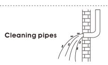
Before installing the faucet, please be sure to remove sundries and sludge from the water pipe to prevent sundries from blocking the faucet.
