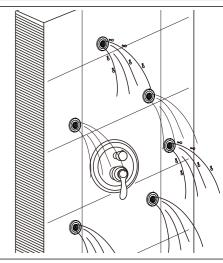
Attach the cover plate to body jets. Apply Teflon tane to threaded tail of the body jets. Use a wrench to screw the jet heads clockwise into the body spray outlets.
