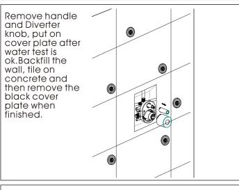
Feed the valve body with panel , handle and diverter , then use the allen key and screw to secure handle and diverter.
