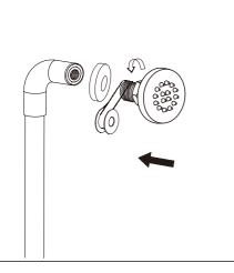
Set the decorative Cup on the shower arm. Roll the teflon tape on the thread. Tighten the shower arm clockwise on the water outlet hole of the shower arm. Then put the overhead shower on the shower arm.
