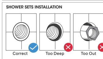
After tiling, the distance from the tile surface to the brass fittings (recessed the wall) is: D:The shower bracket (and bathtub faucet) is 0.4 inch. 2:The shower arm is 0.2 inch.
