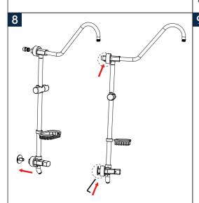
Install the whole product on the wall according to the picture on the right, push the top and bottom two decorative covers outwards, use a hexagonal wrench to tighten the screws clockwise, and then push the decorative cover back toward the wall.
