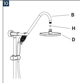
Install the shower head D and the sealing washer H to B as shown in the figure.
