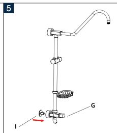
As shown in the picture, insert part I into the corresponding mounting hole of part G (if you cannot insert it, you can use a hexagonal wrench to loosen the screw at the corresponding position of G counterclockwise, and then insert part I).
