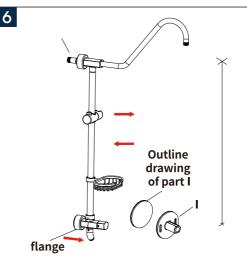
As shown in the picture, push the decorative cover on G in the direction of the arrow to expose part I. Use a horizontal ruler to find the vertical angle, draw the outline of part I and the two screw holes with a pencil, and then remove the entire assembly.
