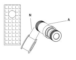
As shown in the picture, wrap the threaded end of part A with Teflon tape 2 times. Screw one end of the thread of Part A into the installation hole of the shower arm in a clockwise direction, and tighten it with a wrench.
