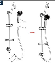
Install the hand shower C. The shower hose M and the two sealing gaskets are as shown in the figure.
