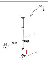
As shown in the picture, insert part G into the corresponding mounting hole of part F, and tighten the nut at the bottom of F clockwise.
