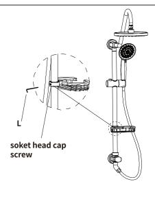
Use the hexagon wrench L to adjust the hexagon socket screws corresponding to the soap basket, and the height of the soap basket can be adjusted according to the user's own needs.
