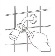
If you have an old shower head, you can remove the top shower with a wrench and insert a screwdriver into the shower arm tube to remove the shower arm.
