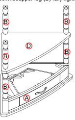
Step 2: Align and place Upper Leg (B) into Table Top (A) then use your hand to rotate clockwise fully tight.
