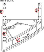
Step 4: Align and place shelf (D) into upper leg (B) and take stand leg (C) into upper leg (B) then use your hand to rotate clockwise stand leg (C) fully tighten.
