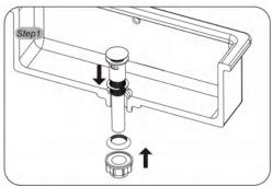
Disassembly part and insert the drain pipe into the hols of basin sink, please sure the samll gasket is above the basin hole, then put and onto the drain pipe;
