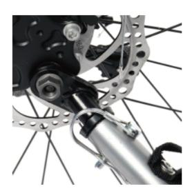
2. You can fix attach the head connector part to the rear end of the bike, with a pin for quick attachment or detachment of the trailer.
