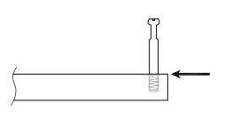
Screw the Cam Screw into the prethreaded hole. Tighten with a screwdriver until snug.
