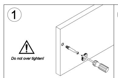
The base of the Cam Screw should be flush with the panel
