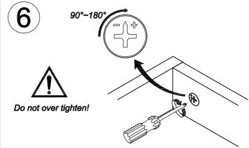
Using a screwdriver, turn the Cam Lock at least 90° clock-wise to lock the two panels firmly togethe.
