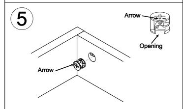
Insert the Cam Lock into the large hole.
