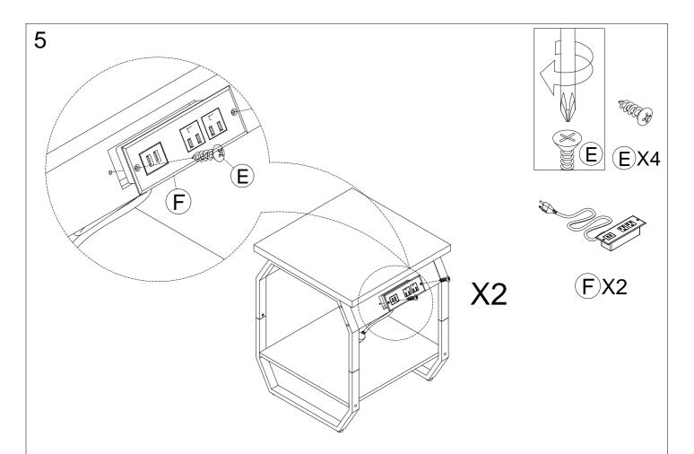
Put hardware F into Part 4 and tighten them with hardware E.
