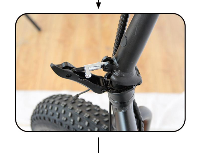
3. Push the lock switch outwards, hold the handle and fold inward immediately
