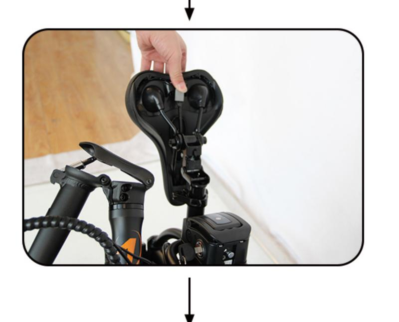
6. Fold the seat cushion, lift the switch under the seat cushion and grab the seat cushion, lift up to fold the seat cushion, turn the battery key counterclockwise to unlock the battery, and take out the battery
