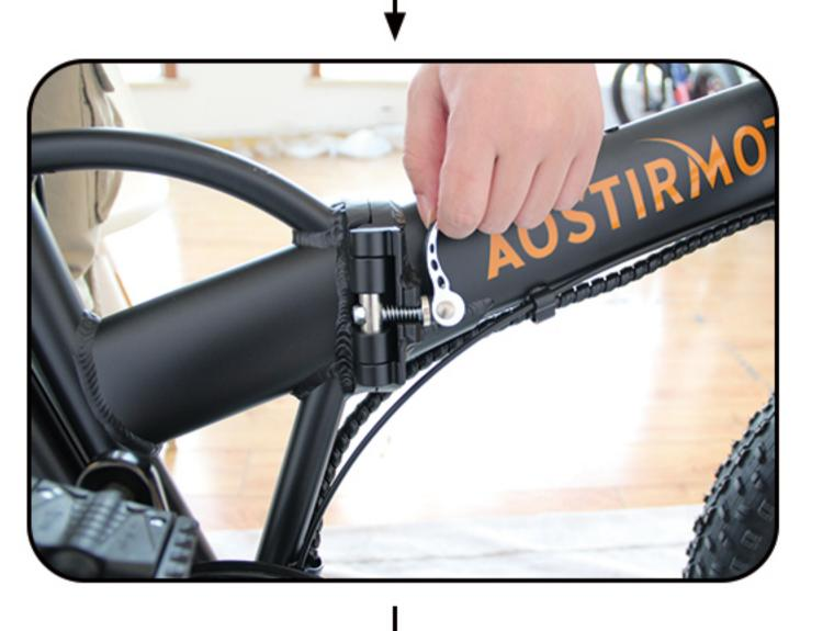
4. Fold the body, push the lock switch upwards, and then turn the switch clockwise
