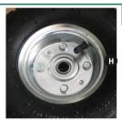
Attach 1x Wheel (H) to one of the axles on either part (B/C) us g 1x washer (f) and 1x pin (e).
