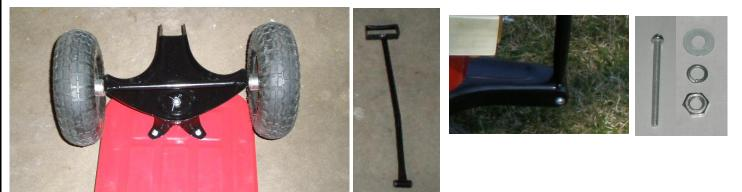
Attach the pull handle (R) to the front axle assembly (S) using bolt (C), flat washer (H), lock washer (J), and hex nut (K). Tighten nut and bolt using flat screwdriver and 10mm wrench. Step 8:
