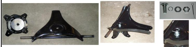
Connect three pieces of front axle assembly (S+I) together using carriage bolt (D), flat washer (N), lock washer (O), grooved hex nut (M) and cotter pin (G). Grooved hex nut needs to only be "finger tight", if over tightened the axle assembly will not turn properly. The cotter pin inserted through the carriage bolt will keep hex nut from backing off the bolt.
