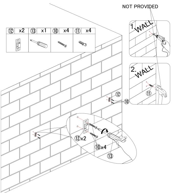
STEP17:Install the anti-collapse device.
