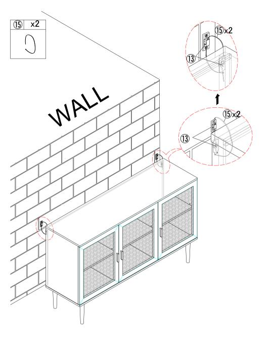
**STEP19:** Let the plastic belt (15) pass through the both part (13) and pull tightly.
