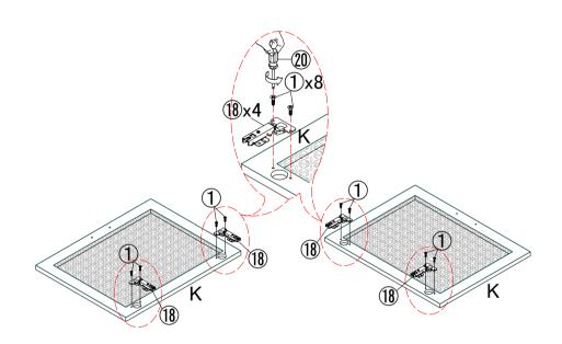
STEP11:Use screw 1 to attach the hinges 8 to door panel (K), tighten screws 1 with screwdriver 20.
