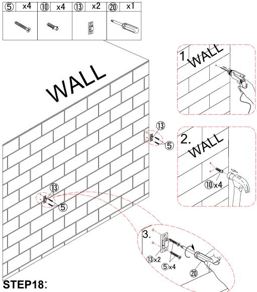
Mark the position on the wall, that corresponds to the location of part (1) on the side panel D&C; Drill and insert the expandable screw (1) by hammer.
