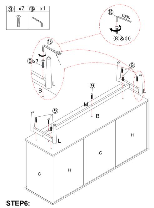
connect the leg frame to the cabinet. Attach the leg frame to the pre-assembled unit in step 4 with a screw (9) and tighten (9) with a allen key (16).
