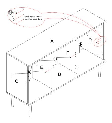
STEP9: Insert shelf pin (4) into pre-assemble unit at step 8.
