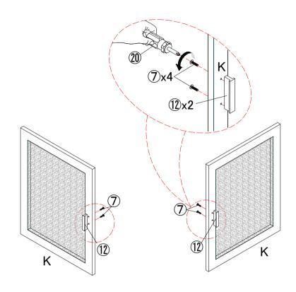
STEP12:Use bolt 7 to attach handle 12 to door panel (K), tighten bolts 7 with screwdriver 20.
