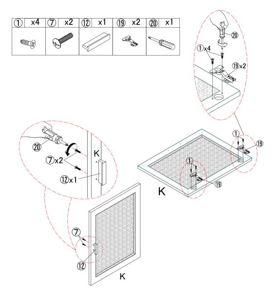
STEP14:Use screw ① to attach the hinges ⑨ to door panel (K), tighten screws ① with screwdriver ⑩.
